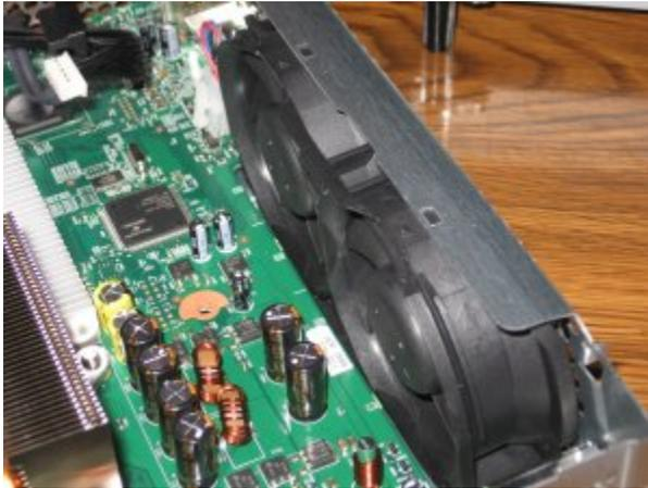
Now go to the front of the console. We need to remove the RF board that contains the power button for the console. Remove the white plastic part of the ring of lights by pulling the bottom clip slightly down with your fingernail, then raising it straight up. You can then remove the three T8 screws holding the RF board in place. Grab the whole board and pull straight out, unplugging it from the console. Set it off to the side.
