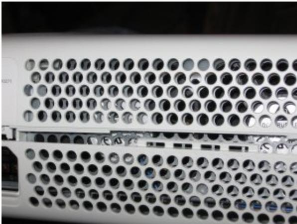
Flip the console over so it is bottom side up and front facing you. You need to remove the Microsoft warranty sticker. You will see four simple tabs holding the front seam together. Simply lift these tabs with a fingernail one at a time until all four are released. You can now remove the top of the case and set it aside.
