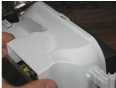
At this point you can remove the fans. Both fans come out in one piece. Unplug the fans from the board. The plug is located just to the left of the fans at the back side of the case. It's a little tight but you can get to it. Squeeze the release clip and lift straight up on the plug. Now put your tool center of the fans at the top between the fans and case. Gently pry up so the fans clear the case. Tilt the top of the fans forward until they clear and lift them straight out.
