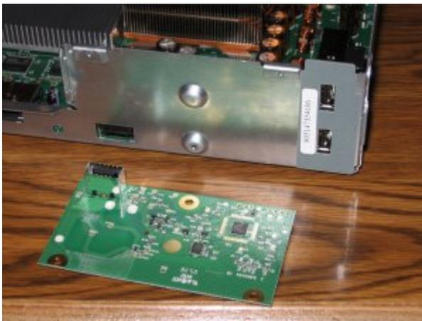
We will now remove the motherboard. Grab the metal USB housing and gently lift up while helping it out with your other hand by lifting on the memory card housings. Once the front is up and clears, just pull the board forward and up.
