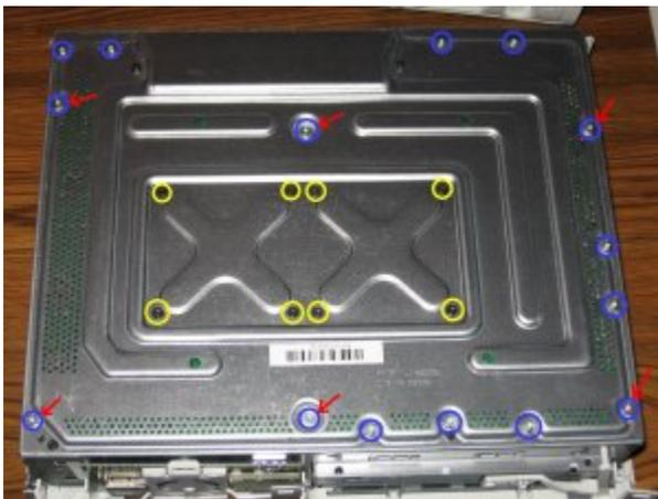
After all the screws are out, simply flip the console back over with the top side up and front facing you again. You can slightly pull the eject button away from the console and lift the top half of the case off and set it off to the side.
