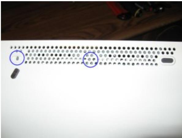
Now flip the console over and do the three clips on the topside. Start with the hidden clip on the top. Being careful not to let the bottom snap back in, pull the grey end away from the Xbox as you go. Once the grey end is loose, set it off to the side as well.
