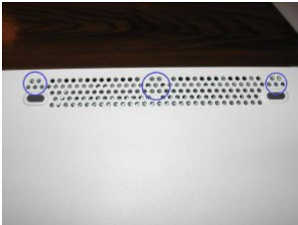
Now flip the console over and do the three clips on the topside. Being careful not to let the bottom snap back in, pull the grey end away from the Xbox as you go.
