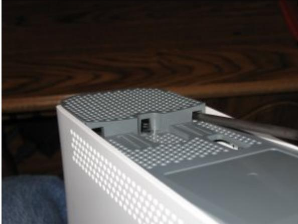
Pull the leftmost rubber foot off (the last tab is only accessible thru the hole under the foot). Release the center tab, then release the one under the foot.
