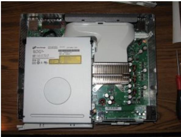
Remove or slice the silver metallic tape holding the front of the DVD drive down. Lift straight up on the drive. Once clear, unplug the power cable and SATA cable. Set the drive off to the side.
